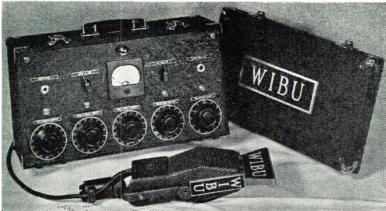
The complete battery-operated remote amplifier as used by radio station WIBU.
